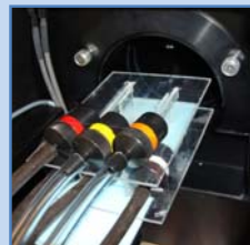
Hoses and nose cones attached to six animal bed in front of the PET/CT bore
